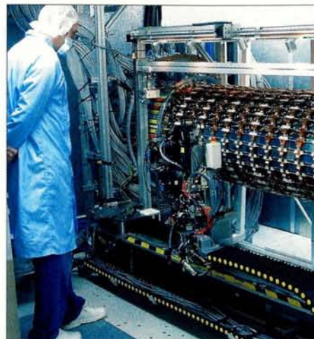
Above: the robot mounts a module on the first barrel of the ATLAS SCT. (Oxford PPU.) Left: the barrel modules are seen more clearly in close-up. (CCLRC.)
