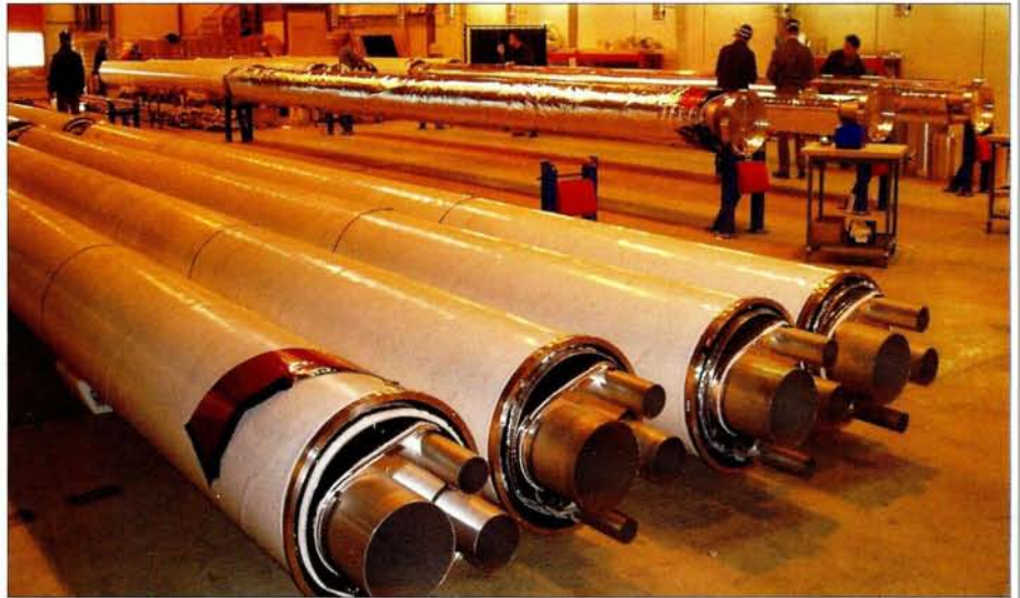
Repair of faulty elements in the cryogenic distribution line is under way at CERN.
