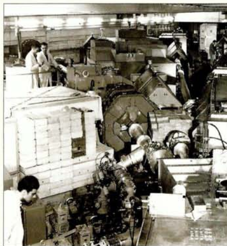
The start of some of the secondary particle beams produced by the 28 GeV proton synchrotron. On the left, shielding bricks form a collimator; to their right are vacuum pipes, passing through guiding lenses and magnets, for beams of charged particles.
