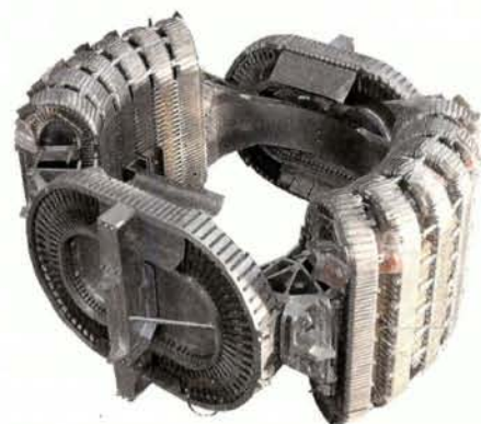
AMS - a 1.1 m clear bore actively-shielded dipole magnet for use in space
